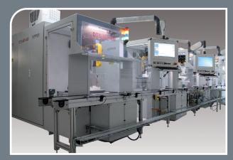
**Electric motor test system** EOL for automotive
