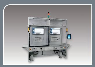
**Trafo test system** Small transformers
