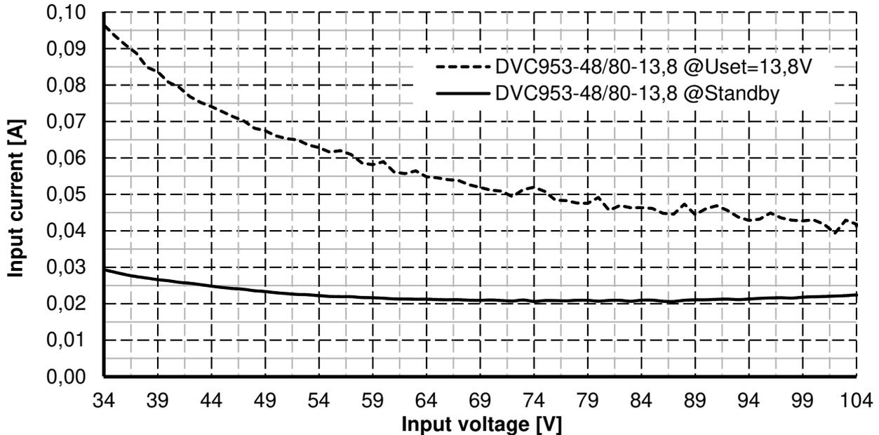
Figure 10.1: No-load current consumption
