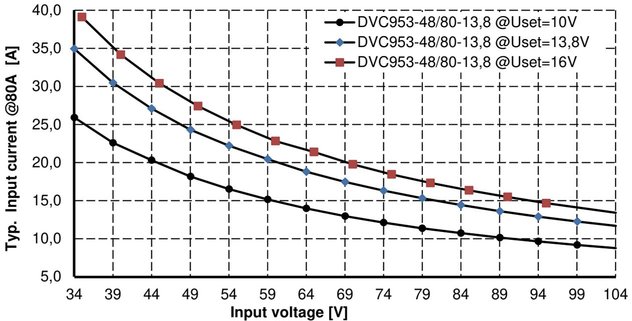
Figure 10.3: current consumption at maximum output current
