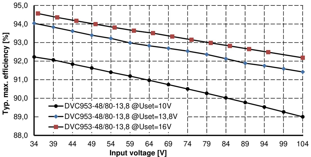
Figure 10.4: Maximum efficiency depending on input voltage
