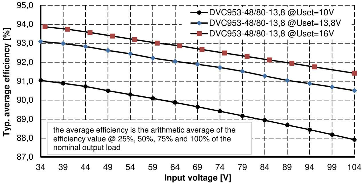
Figure 10.5: Average efficiency depending on input voltage
