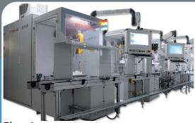
Electric motor test system
